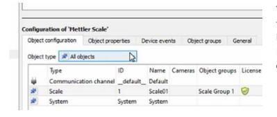
The object configuration tab is where all the individual objects that comprise the integration may be viewed. The Mettler Integration has two object types: Communication Channel and Scale.
