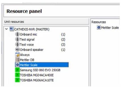
Drag the Mettler device from the **Unit Resources** list into the **Resources** list, on the right.
